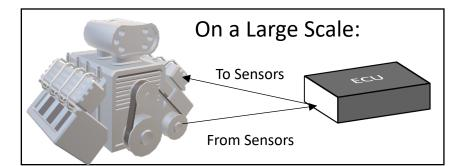
"Harness" is a cable that splits into connections for all the engine sensors/components being used.
